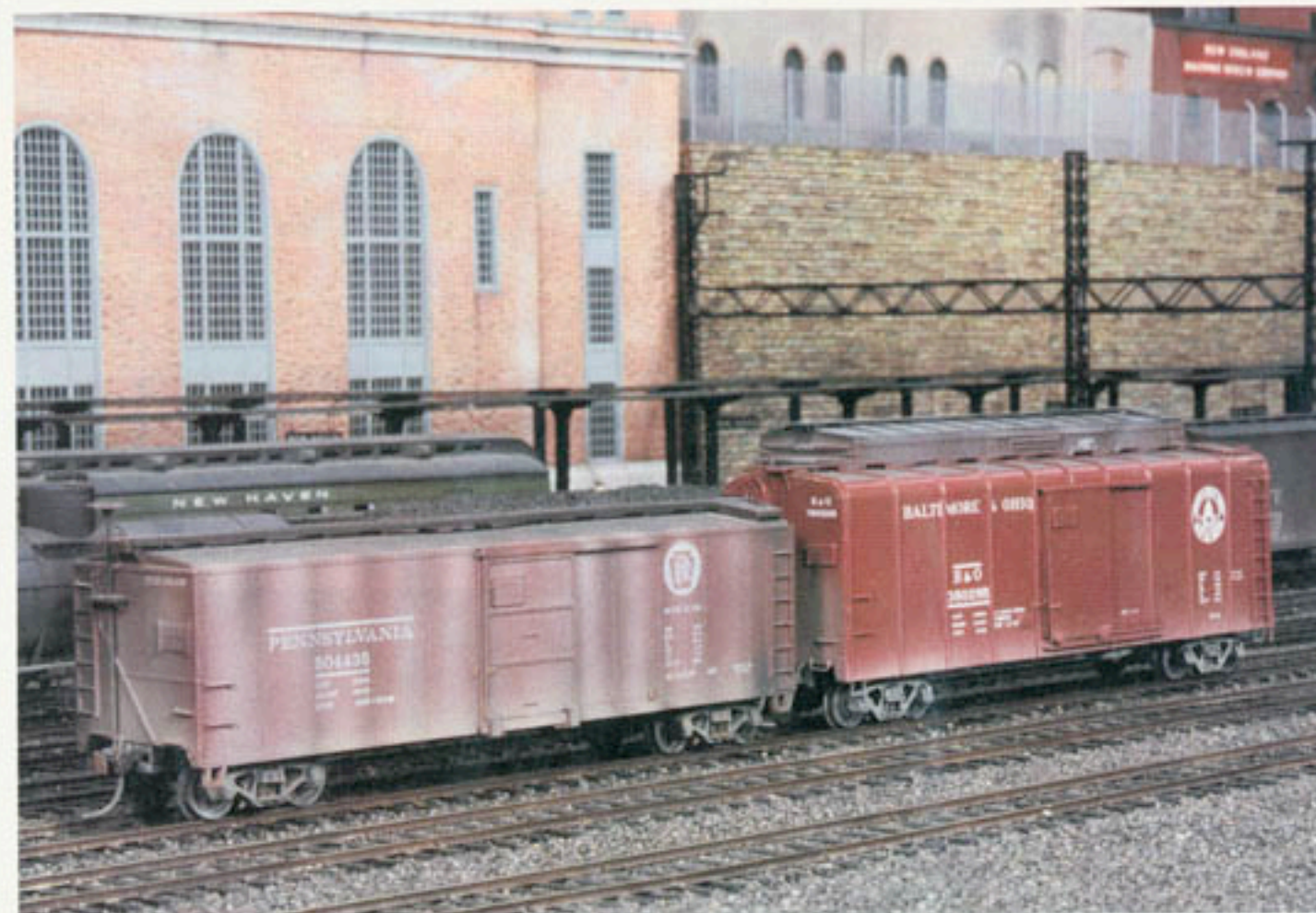
▲ Fig. 4 RIBS AND RIVETS. The Pennsylvania boxcar (left) has light streaks on its panels and dark streaks along its rivet lines. The Pennsy car also has a liberal coating of control coat (Grimy Black diluted 50 percent) to make it look older than the Baltimore & Ohio car (right).
