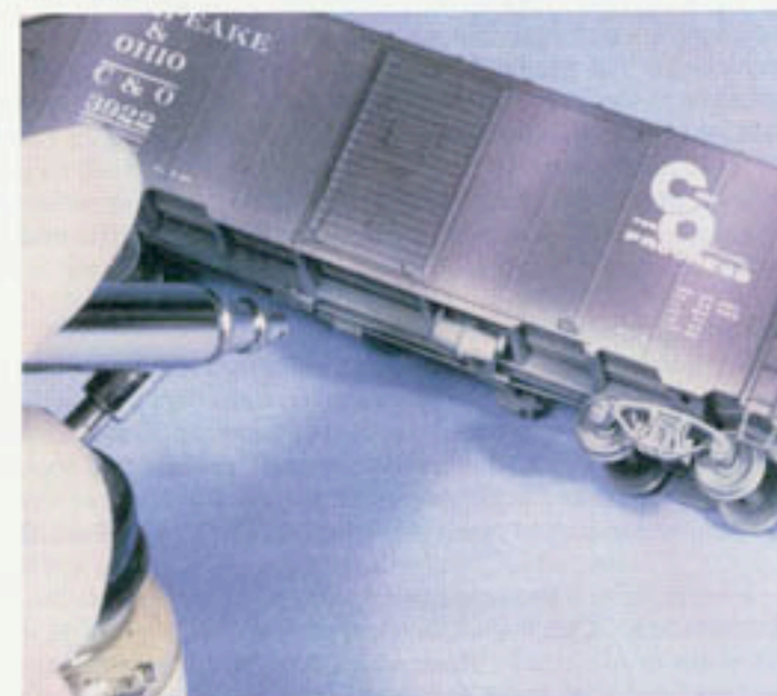
▲ Fig. 5 ROAD DUST. John sprays Earth on the underframe, trucks, and lower portion of the bodies of his cars to simulate dust and dirt kicked up from the roadbed. He changes colors on cars that operate in different regions of North America as shown in table 2.
